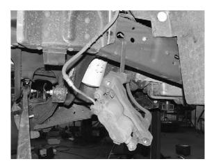
3. Support the I-beam with a floor jack and remove the J clip at the top of the coil spring. Lower the floor jack supporting the I-beams to release the coil spring from the coil bucket and remove the nut at the bottom of the coil spring. Set the coil spring, retaining washer, insulator and lower washer aside. Repeat this on the opposite side. SEE PHOTO BELOW.
