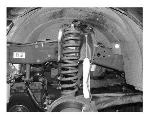
14 Set the truck back on the ground. Reattach the sway bar end links to the I-beams, using the factory hardware. Fully torque the I-beam and radius arm pivot bolts and check all other fasteners. Set the toe-in to approximate factory specs. We recommend driving the truck for approximately fifty miles and then have the truck aligned to factory specs.
