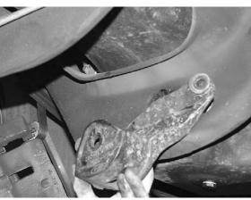
6. Attach the new drop brackets to the frame using the included hardware. You will reuse most of the factory holes and have to drill some new ones. Locate the existing holes with the supplied bolts and mark the new holes that must be drilled with a center punch. SEE PHOTOS BELOW AND ON NEXT PAGE.
