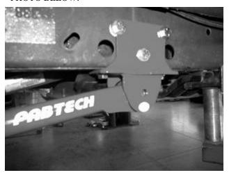
13. Take the **upper link arms** (FT3400-108) and install a grease fitting in each barrel end. Note the offset position of the grease fitting. Lubricating all parts thoroughly with the supplied silicon lube, slide a FT1001 bushing into the barrel with a FT1002 in the opposite side. The offset of the bushings will allow grease to flow through the space between the two bushings. Press a FT3400-102 sleeve into the bushings. Repeat this on each end of both link arms. SEE DIAGRAM ON NEXT PAGE.
