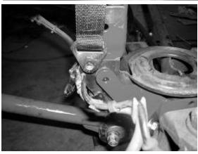
8. Using a ¾" bit, drill out the taper in the track bar frame bracket. Using the supplied ¾" bolt and nut, secure the track bar drop bracket (FT3500-104) to the frame mount and hand tighten the ¾" bolt. Line up the support tube to the frame and torque the ¾" bolt to 100 ft/lbs. Weld the track bar bracket and support tube end to the frame as shown below. After everything has fully cooled, paint all bare metal surfaces. SEE PHOTO IN NEXT COLUMN.
