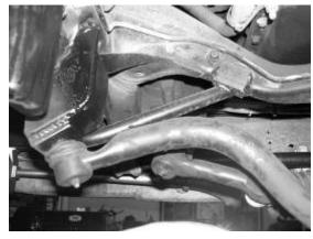
9. Remove the nut securing the pitman arm to the steering box. Using a pitman arm puller, remove the pitman arm from the steering box. Slide the new pitman arm onto the steering box shaft, making sure to line up the splines properly. Reinstall the original lock washer and nut and torque to 220 ft/lbs. SEE PHOTO BELOW.
