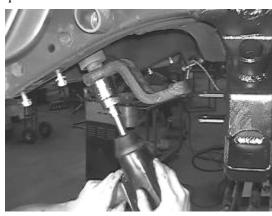
Using a die grinder or sawzall, cut the original lower link arm bracket off of the frame as shown above. Using a sander, grind down any rough edges and remove any paint around the cut surface. Tack weld the supplied weld in plates (FT3400-110) over the cut link arm mount. Completely weld around the plate. After everything has cooled, paint all exposed metal surfaces. Repeat this on the opposite side. SEE PHOTOS BELOW & NEXT PAGE.
