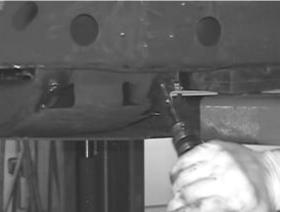
12. Attach the bracket back onto the frame using the supplied ½" x 1 ½" bolts, flat washers and nuts. Torque all hardware to 65 ft/lbs. Repeat this on the opposite side. SEE PHOTO BELOW.
