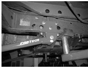
18. Take one of the new coil springs (not supplied with this kit) and locate the top of the coil spring (smaller diameter end). Place the original coil spring insulator on top of the coil spring and place the coil spring onto the front axle. Align the coil spring in the upper and lower pockets and raise the jacks supporting the front axle. Raise the axle just enough to compress the coil spring ½". DO NOT LIFT THE TRUCK OFF OF THE SUPPORT STANDS. SEE PHOTO ON NEXT PAGE.
