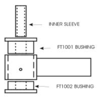
14. Take the **lower link arms** (FT3400-109BK) and install a grease fitting in each barrel end. Lubricating all parts thoroughly with the supplied silicon lube, slide two FT1001 bushings into the barrel. Press a FT97150-6-101 sleeve into the bushings. Repeat this on each end of both link arms. SEE DIAGRAM BELOW.
