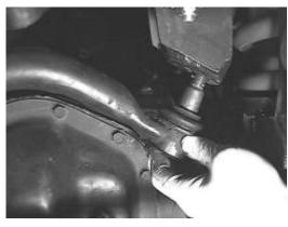
20. Connect the drag link to the new drop pitman arm. Torque the original castle nut to 45 ft/lbs. followed by the proper amount to line up a cotter pin hole. DO NOT LOOSEN THE NUT TO LINE UP THE COTTER PIN HOLE. Install one of the new supplied cotter pins. SEE PHOTO BELOW.
