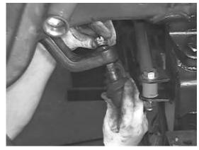
21. Starting on the driver's side of the truck, attach the sway bar drop bracket (FT3400-112D) to the frame in the original sway bar mounting holes using the original bolts. Repeat this on the opposite side using the passenger's side
