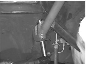
6. Position the lower shock mount below the lower coil spring mount. Secure the bracket to the lower coil spring mount using the supplied ½" x 1 ½" bolts, ½" flat washers and ½" lock nut. You will need to drill out the 2 factory holes to ½". The rear hole will use the ½" x 4 ½" bolt, nut and washer, throw the existing link arm hole. SEE PHOTO BELOW. ( PICTURE IS OF PASSENGER SIDE )
