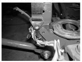
11. Attach the front shock to the mounts using ½" x 3" bolts, with ½" flat washers and a lock nuts. Torque all shock bolts to 40 ft/lbs. SEE PHOTO BELOW AND NEXT PAGE.
