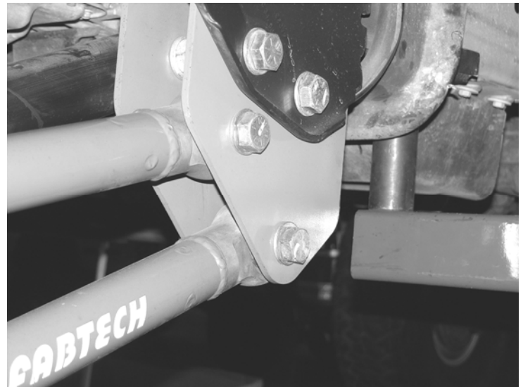
Assembly of the FT292 Alignment Cam
