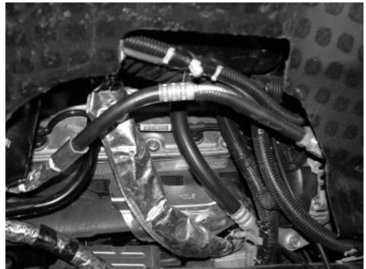
Photo shows bent A/C line
