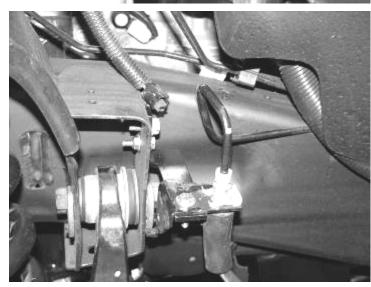
38. Re-route the brake hose and the ABS Line to the steering knuckle using the adel clamp to the back of the steering knuckle and attach with ¼" x 3/4" bolt and washer. Torque to 10 ft lbs. Route the ABS line next to the brake hose. Re-connect the ABS line to the harness in the wheel well. Using provided plastic tyraps secure line to the hose and away from the tire and wheel. SEE PHOTO BELOW
