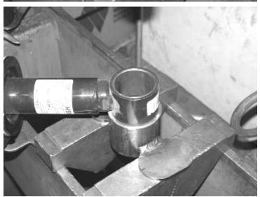
26. Locate Box 3 FTS21042BK which has FT20339 Shock Mount to Arm, FT20323 Shock Extensions, FT20568 Shock Brackets, FT20342 (non auto-ride) or FT20351 (auto-ride) Aluminum Bushings, Hardware Kit FT20295, FT1036 Bushings, and FT148 Sleeves. Using a press, press the bushings and sleeves (Important: must use the provided lube) into the shock extension. Insert the Aluminum Bushings into the bottom of the factory shock. SEE PHOTOS IN NEXT COLUMN
