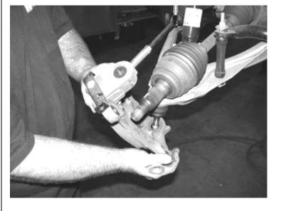
Remove the shock assembly and save with the hardware.
