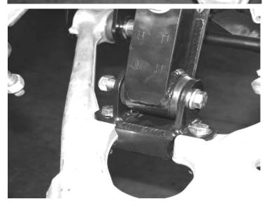
30. Locate the steering knuckle FT20276D and FT20276P. Attach the lower control arm to the knuckle using the stock hardware and torque to 70 ft lbs. Attach the upper control arm to the new knuckle using the factory hardware and torque to 35 ft lbs.
