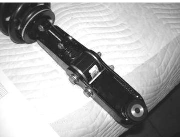
28. Locate the factory upper shock hardware. Install the shock into the factory shock bucket and leave loose. SEE PHOTO BELOW AND ON NEXT PAGE.
