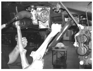
9. Locate, remove, and save the sway bar, discard hardware. SEE PHOTO BELOW
