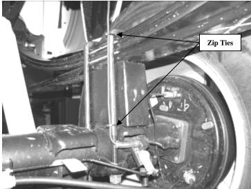
51. Remove the driver's side E-brake cable from the previously removed bracket. Position the passenger side cable into the bottom position of the bracket where the driver's side was originally. Re-install the bracket back into the factory location with the factory hardware. SEE PHOTO BELOW.
