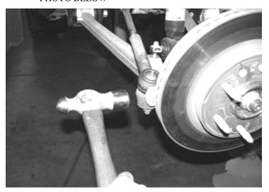
3. Unplug the ABS brake connection from the frame and control arm. Remove the brake hose bracket from the steering knuckle. Remove the brake hose bracket from the coil bucket and save hardware. Remove the caliper from the rotor and secure the brake caliper to the frame out of the way. DO NOT ALLOW THE BRAKE CALIPER TO HANG FROM THE BRAKE LINE HOSE. SEE PHOTO BELOW
