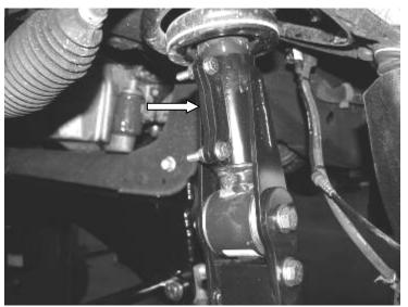
Photo shows new style shock brackets
