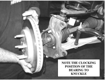
5. Remove the upper and lower ball joint nuts. Disconnect the upper and lower ball joints from the steering knuckle by striking the knuckle with a large hammer next to each ball joint on the knuckle to dislodge the ball joints. Use care not to hit the ball joints when removing. Save nuts and discard knuckle. SEE PHOTO BELOW
