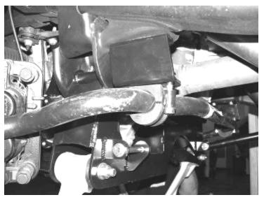
36. Locate FT20602 Sway Bar Mounts and the supplied 18mm x 50mm hardware. Position the Sway Bar Mount so that it is on the bottom of the sway bar with the SHORTER side of the mount against the stop plate end of the mount. Attach with the 18mm hardware and torque to 110 ft lbs. Locate the factory sway bar end links and attach to the new mount and the lower control arm. SEE DIAGRAM BELOW.
