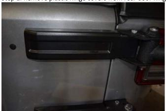
Step 2: Remove the two 13 mm bolts from upper hinge on the rear door. (note: Only do 1 hinge at a time)
