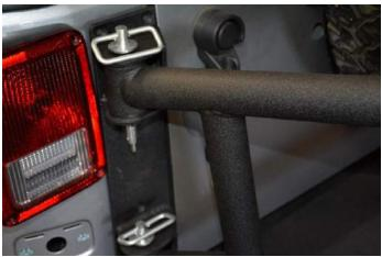
Step 17: With the tire carrier in the closed position and the new body bracket touching the rear body panel take a marker and mark the 5 mounting hole locations.
