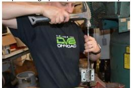
Step 6: Pull the hinge apart and discard the portion of the hinge that previously bolted to the body.
