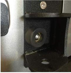
Step 22: Tire carrier adjustment up or down to ensure proper alignment with rear body plate. The upper body hinge has an adjustable cam, turn clockwise or counter-clockwise to move tire carrier up or down. Once you have centered the tire carrier so that it engages smoothly with the body plate secure hinge bolts and tighten.
