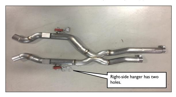
7. Install the 2 clamps onto the front pipes. Note that the bolts are on the left-side of the pipes, and the nuts are facing downward.
