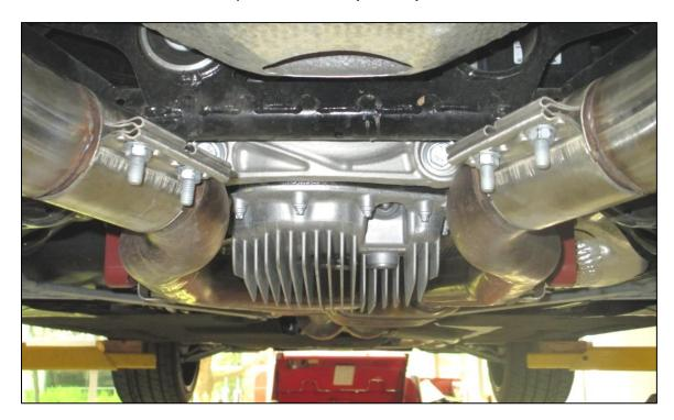
14. Check the exhaust tips for proper bumper clearance and alignment per the photos below.
