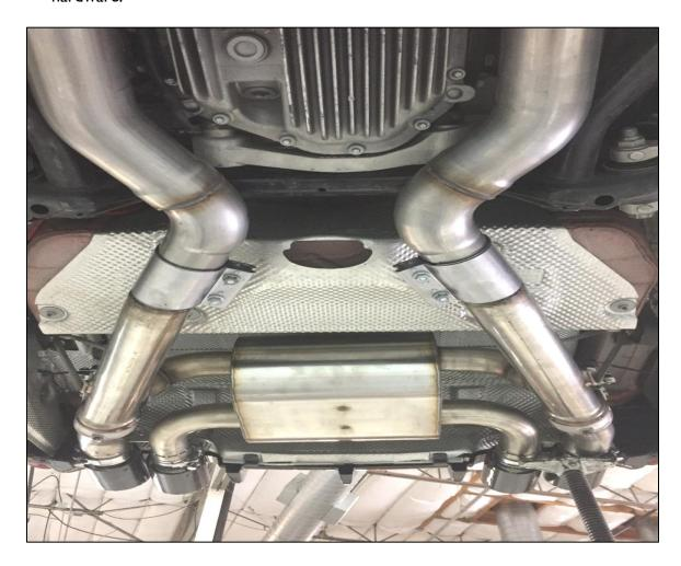
11. Adjust fitment to obtain 1/4" clearance between the heat shield and the left-side pipe near the fuel tank. This clearance will naturally increase when the exhaust gets hot.
