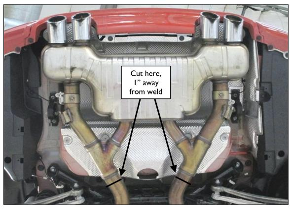
5. Remove the two nuts and one bolt that hold the hangers to the subframe, and remove stock midpipe from car.
