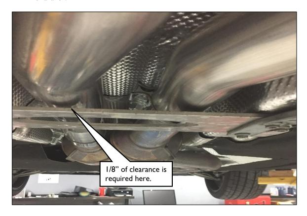
• If after adjustment, further clearance is needed -- install spacer plate between cross brace and body to obtain additional clearance.
