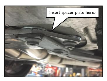
16. Drive car and get the exhaust hot. Recheck for adequate clearance in all areas. If necessary, let pipes cool before performing further adjustment. Re-torque all the clamps.
