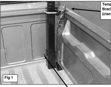
Temporarily clamp Bracket to vehicle (clamp not included)
