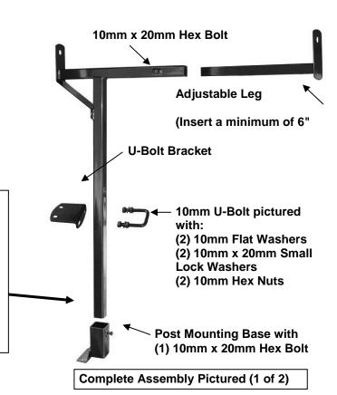
The Universal Ladder Rack height can be adjusted to fit a variety of vehicles. Determine the desired height, (leave a minimum 3" of clearance above the top of the cab), and cut off the bottom of the (2) Main Posts. **NOTE:** Cutting the Main Posts will damage the powder coated finish. Paint the exposed bare metal to resist rust.
