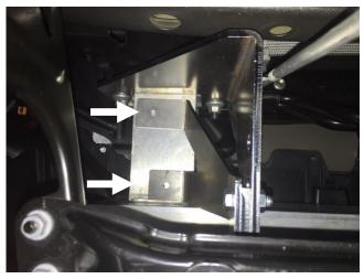
**Step 4**: After light bar is properly adjusted, tighten all hardware.
