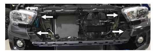
**Step 5:** Remove the plastic fog light trim piece by pulling forward to release the six pins (both sides)
