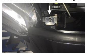
**Step 3:** Carefully left the two support brackets enough to clear the mounts.
