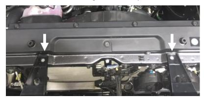
Step 2: Next remove the two push pins located on the left and right side of grill.
