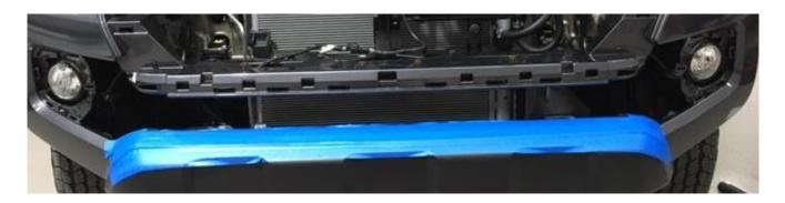
**Step 8:** Remove the plastic side cover by releasing the push pin and pulling forward from the clip. (both sides)
