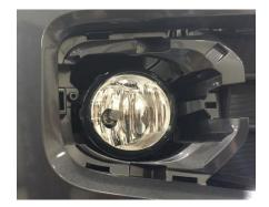
**Step 6:** Using a panel tool or flat head screw driver, release the 23 pins holding the plastic insert to the bumper.
