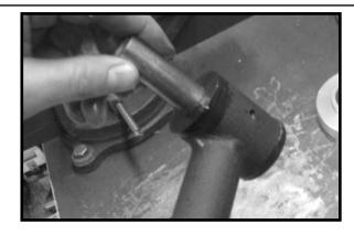
25. Locate the new sert fittings from hardware bag 54060PL Install the new sert fittings into the new upper control arms. Special note: Make sure not to over tighten and also make sure that the sert fitting is facing towards the outside of the vehicle. This will make for easier access when using a grease gun.
