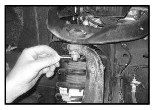
8. Working on the driver side, loosen but do not remove the castle nut holding the upper control arm to the knuckle. With a hammer, carefully hit the knuckle to break the taper. Once the taper has been broken, remove the castle nut and discard. Separate the upper control arm from the knuckle. Repeat procedure on the passenger side.
