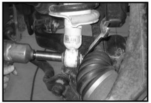
Tuff Country EZ-Ride Suspension recommends a wall mounted strut compressor be used when performing the steps that talk about installing the pre-load spacer into the strut. If you do not have a wall mounted strut compressor, please have these steps performed by your local Nissan Dealership
