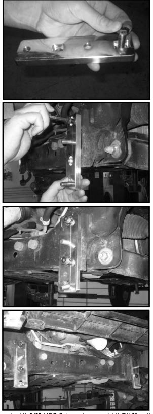
5. Locate (4) 3/8" USS flat washers and (4) 7/16" unitorque nuts from hardware bag 54060NB. Working on the driver side, attach the sway bar to the newly installed sway bar (4) 7/16" x 1 1/4" bolt and (4) 12 mm x 30 mm socket head bolts from hardware bag 54060NB. Install the new 7/16" x 1 1/4" bolts to the new sway bar brackets into the cut out slot.
