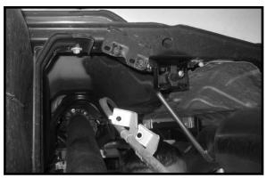
spacer sleeve between the brake line and axle and secure 45. Locate (2) emergency brake line relocation brackets using the new 8 mm bolt and hardware. Make sure to use from hardware bag 54060NB1. Install the new brackets to loctite and torque to 12 ft lbs. the OE location using the OE hardware. Make sure to use
