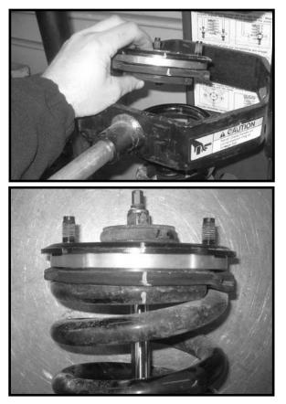
19. Locate the new upper strut spacer. Install the new upper strut spacer to the modified strut and secure using the OE hardware. Make sure to use loctite and torque to **45 ft. Ibs.** Place the driver side strut aside for later installation into the vehicle.
