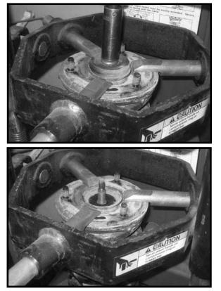
16. Carefully loosen the wall mounted strut compressor until the bearing plate can be removed from the coil over.
