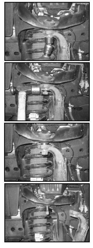
9. Working on the driver side, remove the hardware attaching the upper control arm into the OE pockets. Save the OE hardware but the control arm may be discarded. Repeat procedure on the passenger side. **Special note: On the driver side only, the brake line will need to be removed from the bracket so that the rear upper control arm bolt can be removed. Save the brake line hardware.**
