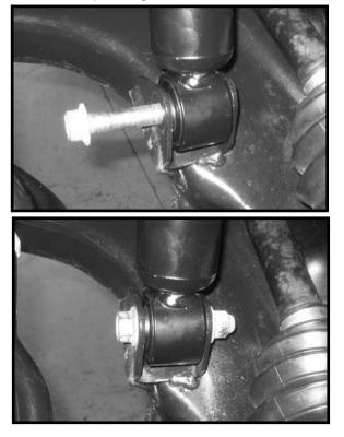
23. Working on the driver side, move back to the 3/8" hardware and add some loctite and torque the (3) nuts to 28 ft **Ibs.** Repeat procedure on the passenger side.
