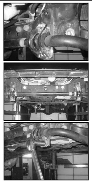
6. Place a pair of hydraulic floor jacks under the driver and passenger side lower control arm. Carefully raise up on both hydraulic floor jacks until they come into contact with the lower control arms.
