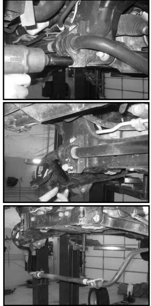
Working on the driver side, install the new bracket to the OE location and secure using the new 12 mm x 30 mm socket head bolts. Make sure to use loctite and torque to **40 ft lbs.** Repeat procedure on the passenger side.
