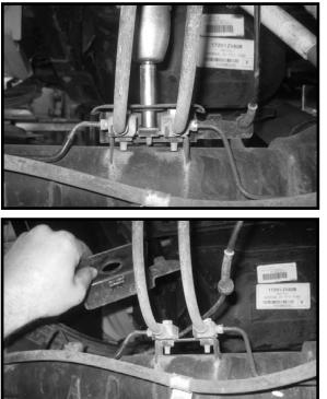
41. Working on the rear axle, remove the brake lines from the OE mounting location. The hardware may be discarded.
