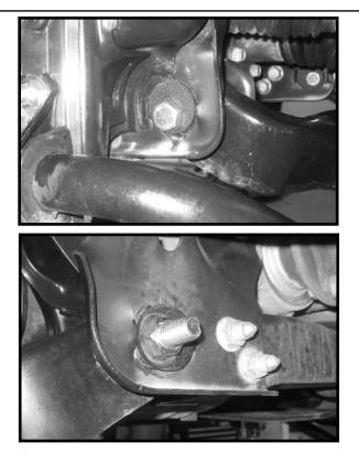
33. Locate (2) S10066 spacer sleeves from hardware bag 54060NB1. Also, locate (2) 6 mm x 70 mm bolts, (2) 6 mm lock washers and (2) 1/4" fender washers from hardware bag 54060NB. Secure the rear portion of the skid plate to the OE location using the new spacer sleeve and hardware. Make sure to use loctite and torque to **8 ft lbs.**
