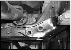
9. Locate the new rear long arm bracket and (2) cross member bracket shims. Locate (2) 9/16" x 8" bolts, (4) 1/2" USS and (2) 1/2" unitorque nuts from hardware bag 30940NB1. flat washers and (4) 9/16" unitorque nuts from hardware bag 30940NB1. Working on the driver side, install the new rear long arm bracket to the new location on the frame and the side of the transmission cross member. Secure using the torque to **55 ft lbs.**
