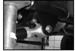
19. Locate the stock cam bolts and hardware. Install the new longer lower control arm to the axle mount and secure using cam bolts and hardware. For now, center the cam bolt and torque to **95 ft lbs.** Move back to the new mounting hardware that is securing the new longer lower control arm to the rear mount and add some thread locker or loctite and torque to **95 ft lbs.**
