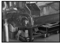
and secure using the new 9/16" x 4" bolt and hardware. **Do not tighten at this point.** Now install the upper control arm to the tabs on the new longer lower control arm and secure using the new 9/16" x 4" bolt and hardware. Add some thread locker or loctite on the new upper control arm hardware and torque to **95 ft lbs.**
