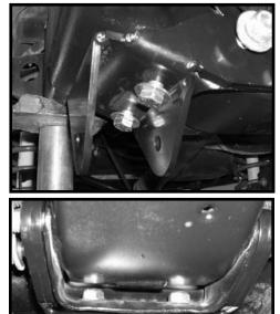
12. Working on the driver side, move back the new 9/16" x 8" bolts holding the legs of the new bracket to the transmission cross member and add some thread locker or loctite and torque to **85 ft lbs.** Now remove the hydraulic floor jacks from under the transmission cross member.
