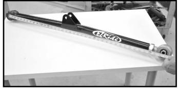
17. Locate (2) 9/16" x 4" bolts, (4) 1/2" USS flat washers and (2) 9/16" unitorque nuts from hardware bag 30945NB Working on the driver side, install the new longer lower con-
