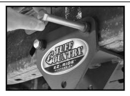
8. Working on driver side and using the newly installed frame bracket as a guide, carefully drill (2) 1/2" holes into the transfer case cross member. Repeat procedure on the passenger side.
