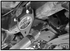
9. Locate (4) 1/2" x 1 1/2" bolts, (8) 7/16" USS flat washers and (4) 1/2" unitorque nuts from hardware bag 30945NB. Working on the driver side, secure the newly installed frame bracket to the transfer case cross member using the new 1/2" hardware. **Do not tighten at this point.** Repeat procedure on the passenger side.
