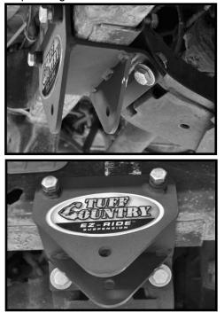
10. Working on the driver side move back to the new 1/2" hardware and add some loctite and torque all 4 bolts to **75 ft Ibs.** Repeat procedure on the passenger side.
