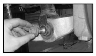
11. Working on the driver side, install the lower control arm into the front and rear lower control arm pockets using the OE hardware. Make sure to use loctite, refer back to the marks that were scribed on the cam washer and cam stops and torque the front and rear mounting hardware to 105 ft lbs. Repeat procedure on the passenger side.
