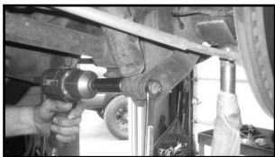
20. Working on the driver side, remove the sway bar end link from the sway bar. Save the hardware and repeat procedure on the passenger side.
