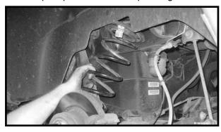
23. Locate the new rear coil springs spacers. Also, locate (2) 7/16" x 1 1/2" bolts, (4) 3/8" USS flat washers and (2) 7/16" unitorque nuts from hardware bag 32102NB. Working on the driver side, install the new 7/16" bolt into the upper coil spring bucket. Hole provided. Then install the new rear coil springs spacer into the upper coil spring bucket and secure using the new hardware. Make sure to use loctite and torque to 42 ft lbs. Repeat procedure on the passenger side.
