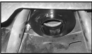
24. Working on the driver side, install the coil spring back into the OE location. Make sure that the OE rubber isolator is installed with the coil spring. Carefully raise up on the hydraulic floor jack until the coil spring seats properly into the lower axle. Repeat procedure on the passenger side.
