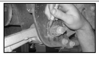
6. Working on the driver side, remove the hardware that attaches the lower control arm to the front and rear lower control arm mounts. Save the hardware. Repeat procedure on the passenger side. **Special note: Let the lower control arms hang and rest on the hydraulic floor jacks.**
