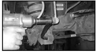
tite and torque to 85 ft lbs. Repeat procedure on the passenger side. The OE rear shocks will be long enough and order your new rear shocks. Tuff Country recom-customer picks up their vehicle. mends install a 26" fully extended nitrogen gas shock.
