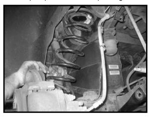
25. Install the track bar to the OE track bar mount and secure using the OE hardware. Make sure to use loctite and torque to **85 ft lbs.**
