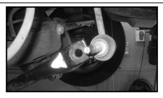
21. Working on the driver side, remove the track bar from the track bar location. Save the hardware.
