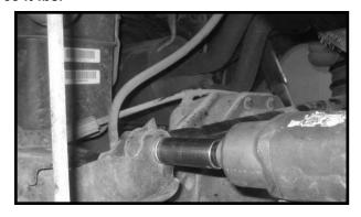
26. Working on the driver side, install the end link to the sway Congratulations, installation complete! bar and secure using the OE hardware. Make sure to use loctite and torque to 40 ft lbs. Repeat procedure on the passenger side.
