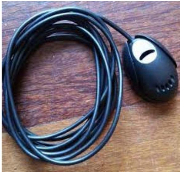
This external mic will work at just about any location, but we do have some recommendations as to placement. Try to keep this mic away from any windows, air vents, or speakers to avoid background sounds or feedback. The external mic will plug into the back of the JK1001 via a 3.5mm headphone jack plug located just to the left of the RCA pigtail. Most folks place this directly on the steering column.
