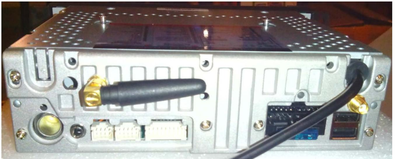
Your Wi-Fi antenna will screw on as shown above. Along with that, your GPS plug in is now on the far right hand side of the JK1001.
