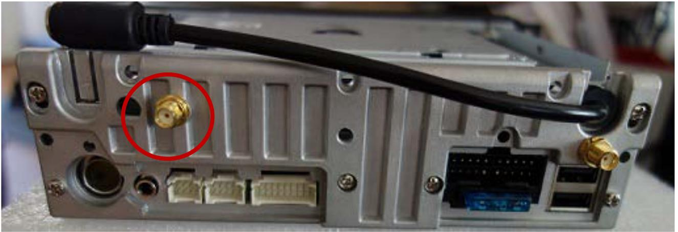
Above is a picture of the back of your JK1001. If your JK1001 is equipped with a Wi-Fi antenna, then you will have this additional gold plated plug just above the RCA plug in.
