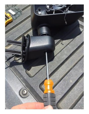
14) Remove all components from the factory housing and set the factory upper plastic portion of the housing aside, you will be reusing the all interior components and the lower plastic piece.
