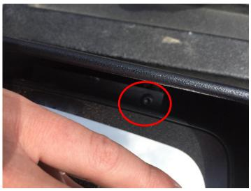
10) Remove the bolt holding the top and bottom portion of the mirror assembly.
