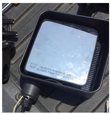
17) Feed all of the wires through the plastic lower housing and then through the lower metal portion in the factory location. (There is a groove cut for them)
