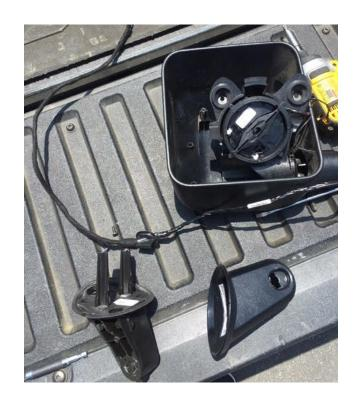
15) Reverse the steps used in step 9 to install the motor mechanism into the new DV8 housing. Install the 3 original bolts back in and feed all wires through the bottom of the new housing.
