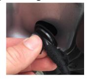
6) Remove the seal plug from the door and proceed to step #7
