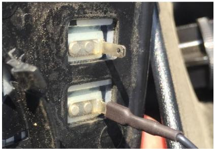
12) If equipped, remove the mirror heater wires from the mirror by simply pulling the connectors apart gently.
