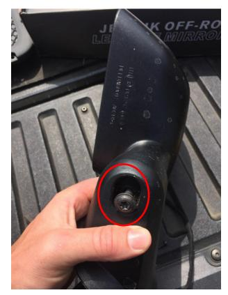
11) Tilt the reflective part of the mirror all the way to one side and locate the clips holding the reflective part of the mirror to the motor mechanism. Using a screwdriver push up on these clips and the mirror will release. Don't use too much force or you risk breaking the mirror. (And 7 years of Bad Luck!)
