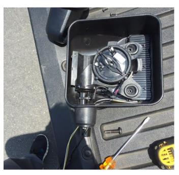
16) Reconnect the heating wires that you removed in step 12, and snap the mirror back into place. Make sure to be gentle in this process.
