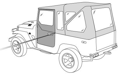
**Note:** If a hard door striker is present, it must be removed. **Note:** Some vehicles will use the existing holes and bolts from the hard door striker.
