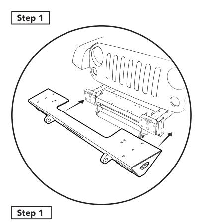
Re-Attach the Front Bumper. The studs on the inside of the Bumper will fit through the holes in the bumper mounting plates and through the holes in the Inner Roller Brackets.
