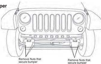
NOTE If you intend to install a winch only, you may install it directly on your bumper and do not need to use the Fare Lead Plate.
