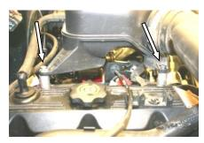
**6.** Install the two 1" aluminum spacers (#5) and provided 6mmx40mm bolts (#6) under the mounting tabs that hold the factory resonator to the top of the valve cover as shown.
