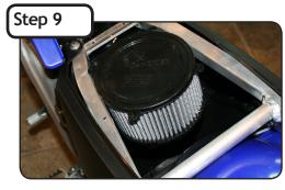
Install the outer Pro DRY S filter onto the inner filter.
