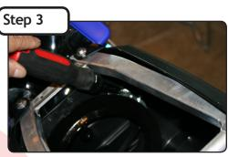
Using a 4mm allen wrench, loosen the clamp around the air boot flange.
