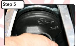
Install the aries AE2 intake tube into the air boot flange. Start with the bottom of the tube and push up toward the top.
