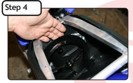
Carefully pry the plastic foam air filter mount out of the air boot flange. You should be able to remove the mount with your fingers.
