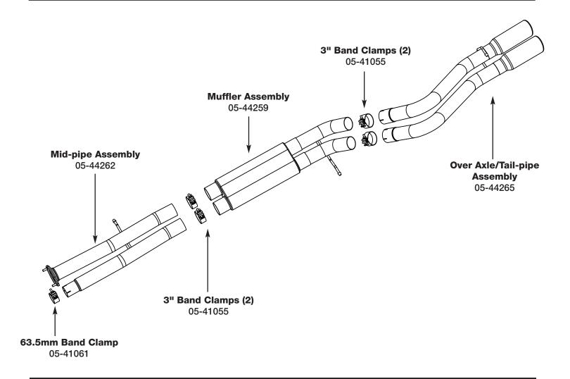
**Step 1:** (Read Instructions prior to installation) Remove your stock exhaust from the rear of your truck working your way forward, it will be necessary to cut the stock exhaust at a convenient location due to it length. Take caution not to damage the factory isolation mounts as they will be reused. It is recommended to not fully tighten the clamps until the entire system has been installed.
