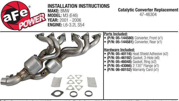
Caution: aFe recommends professional installation on our products. Allow time for your vehicle to cool down prior to installation. When working on or under your vehicle proceed with caution. Exhaust systems reach high temperatures and may cause serious burns. Wear protective safety equipment; eye goggles and gloves to ensure a safe installation.
