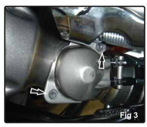
6. Locate the exhaust valve controller at the rear of the fuel tank and remove the exhaust valve controller by removing the one nut holding it in place. Remove the shield and cables from the exhaust controller. Remove the exhaust valve cables from the motorcycle. Reinstall the shield and exhaust valve controller back into the stock location (see Fig 5).
