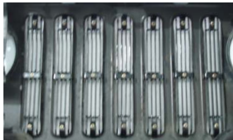
Figure 3 – Rear view of vehicle's shell; Billet Grilles attached with Metal Brackets and Flange Nuts
