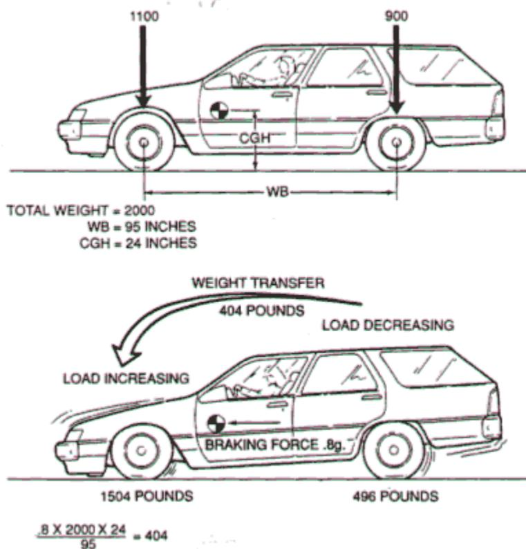
shock absorber or strut performance. Shock absorbers and struts help maintain vertical loads placed on the tires by providing resistance to vehicle bounce, roll and sway during weight transfer. They also help reduce brake dive along with acceleration squat to achieve a balanced ride.
