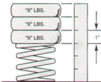
Spring rate, sometimes referred to as deflection rate, is used to measure spring strength. It is the amount of weight that is required to compress the spring 1 inch. For example: If it takes 100 lbs. to compress a spring 1 inch, it would take to 200 lbs. to compress the spring 2 inches.
