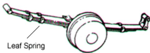
**Leaf Springs** Leaf springs are designed two ways: multi-leaf and mono-leaf. The multi-leaf spring is made of several steel plates of different lengths stacked together. During normal operation, the spring compresses to absorb road shock. The leaf springs bend and slide on each other allowing suspension movement.
