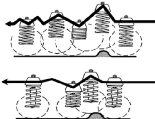
When the spring is deflected, it stores energy. Without shocks and struts the spring will extend and release this energy at an uncontrolled rate. The spring's inertia causes it to bounce and overextend itself. Then it re-compresses, but will again travel too far. The spring continues to bounce at its natural frequency until all of the energy originally put into the spring is used.
