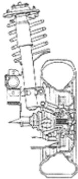
Now that we have a more thorough understanding of shock design, let's focus on the strut. The strut is a common damper type used on many of today's independent suspension, front wheel drive vehicles as well as some rear wheel drive vehicles.
