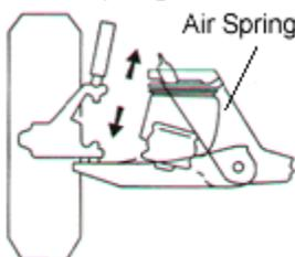
the vehicle load changes, a valve at the top of the airbag opens to add or release air from the air spring. An onboard compressor supplies air.
