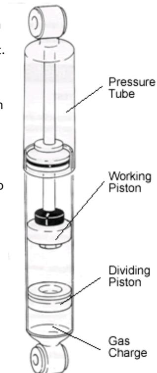
The area below the dividing piston is pressurized to about 360 psi with nitrogen gas. This high gas pressure helps support some of the vehicle's weight. The oil is located in the area above the dividing piston.
