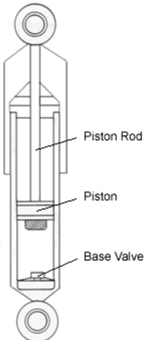
Let's start our discussion of shock absorbers with one of very important point: despite what many people think, conventional shock absorbers do not support vehicle weight. Instead, the primary purpose of the shock absorber is to control spring and suspension movement. This is accomplished by turning the kinetic energy of suspension movement into thermal energy, or heat energy, to be dissipated through the hydraulic fluid.
