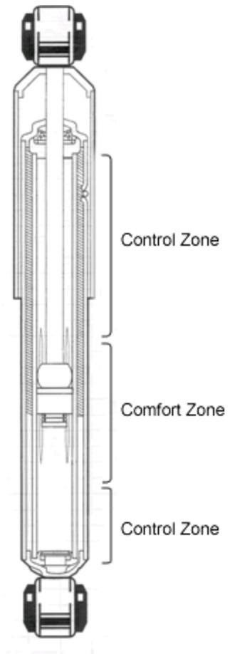
a new compression valve design. This compression valve is a mechanical closed loop system, which opens a bypass to fluid flow around the compression valve.
