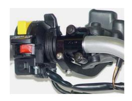
Right side view of ATV, bracket is positioned under brake lever and angles toward center.
