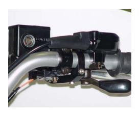
Rear view of ATV throttle, mount bracket is positioned under brake lever.
