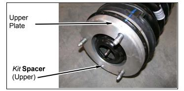
b. From CL230BAG: Install coil-over onto upper perch with three *kit* washers (10mm) and three *kit* nuts (10mm stover) and *kit* Loctite®. TORQUE to OE specification.
