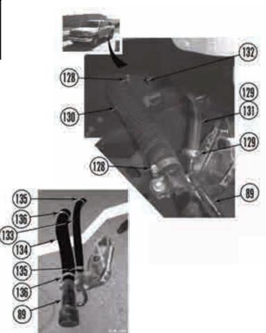
e. Install fuel filler neck (89) on bed (87) with two nuts (88).
