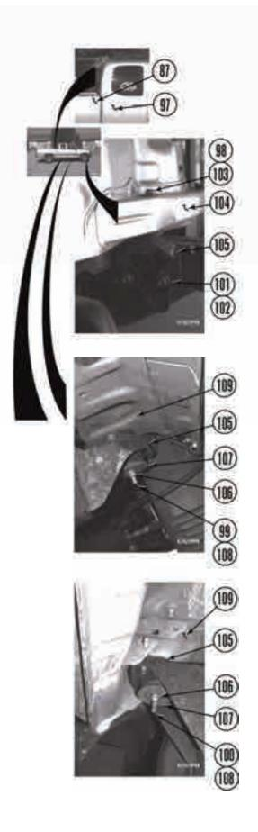
2. Lift cab and install cab passenger side spacer blocks.
