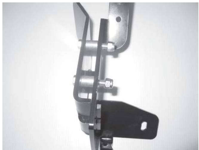
Figure 3 Install bolts and bronze spacers to bracket
