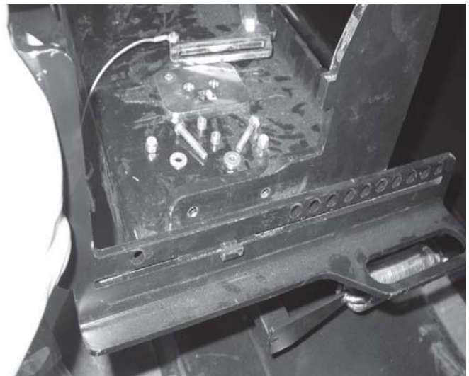
Figure 19 Install stand slot to plow support tab
