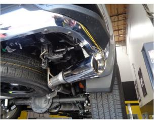
**Step 6.** Using the supplied rubber insulators install the Tailpipe Assemblies to the Extension pipes fitting the hangers into the installed hanger brackets. Finish by attaching the Tips using the supplied 2.75" clamps. Tips can be adjusted to fit a variety of bumpers.
