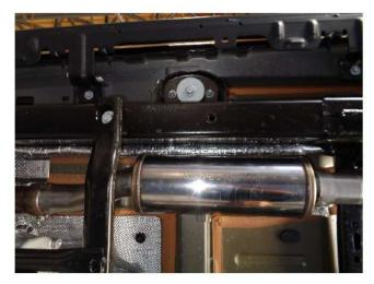
**Step 3:** Begin installation of your new MAGNAFLOW system by attaching the Resonator Assembly to the catalytic converter outlet using the OEM clamp. Engage the welded hanger to the rubber insulators. Keep all fasteners and clamps loose until final adjustment.
