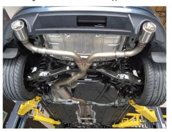
**Step 4.** Next attach the Y-Pipe Assemby to the Muffler Assembly using the supplied 3.00" clamp. Install the two Tail Pipe Assemblies in a similar fashion using the supplied 2.50" clamps. Locate the welded hangers to the rubber insulators.
