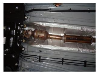
Step 2: Begin installing your new system by sliding the Resonater Assembly over the cut pipe and loosley attaching with the provided 2.38" clamp. Engage the hanger to the rubber insulator.
