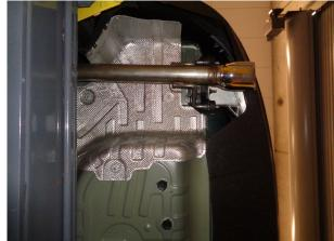
Step 3: Next loosely fasten the Extension Pipe to the Resonator Assembly using the supplied 2.25" clamp. Then attach Tail Pipe Assembly in a similar fashion engaging the welded hangers to the rubber insulators.
