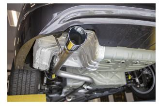
Step 4: Once a final position has been chosen for the new exhaust system, evenly tingten all clamps from front to rear using the torque specifications on page one of these instructions. Inspect all fasteners after 25-50 miles for operation and re-tighten if necessary.
