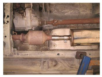
**Step 2.** Install the new system by attaching the new muffler assembly to the catalytic converter using the supplied 2.50" clamp and by locating the welded hanger to the rubber isolator. Be sure to align the locating notch in the muffler pipe with the indexing peg on the OEM system. Leave all clamps and fasteners loose for final adjustment of complete system.
