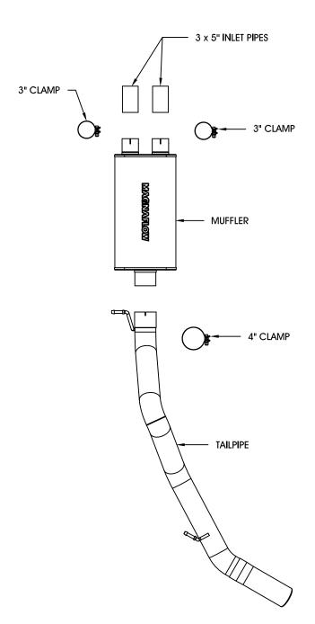
**Warning**: Professionally welded installation of this Magnaflow Performance exhaust system is required.
