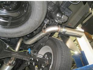
**Step 4.** Next use the supplied 2.50" clamp to attach the Muffler Assembly to the Inlet Pipe. Finish by attaching the Tailpipe Assembly to the Muffler Assembly with the Supplied 3.00" clamp and fitting the hangers into the insulators.
