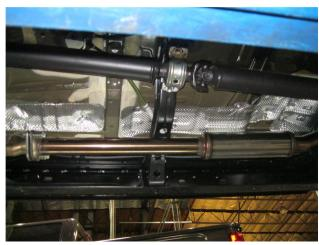
**Step 3.** Begin installation of your new MAGNAFLOW system by attaching the Resonater Assembly to the catalytic converter outlet using the OEM fasteners and insulator. Keep all fasteners and clamps loose until final adjustment.
