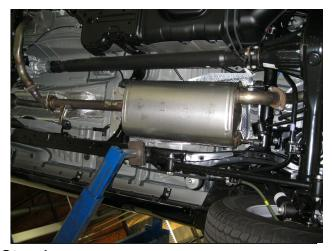
**Step 1.** Begin removing the OEM exhaust by unbolting the spring loaded coupling flange at the outlet of the OEM Y-Pipe that attaches to the muffler inlet with a 14mm socket.
