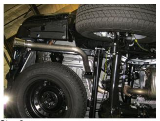
**Step 2.** Next unbolt the outlet of the OEM muffler at the inlet of the tail pipe assembly. Remove the welded hangers from the rubber insulators using a pry bar. do not discard or damage the insulators as they will be needed to install your new system. The OEM system may now be removed.
