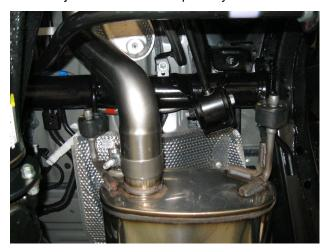
**Step 4.** Slip the inlet of the Muffler Assembly over the outlet of the Inlet Pipe Assembly and loosely secure using the supplied 2.50" clamp and 15mm socket. Engage all welded hangers to the OEM rubber insulators. Install the Mid Pipe and the Tail Pipe Assembly using a similar procedure.
