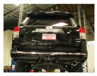
**Step 9.** Once a final position has been chosen for the new system, evenly tighten all fasteners from front to rear using the torque specifications on page one of this document. Inspect all fasteners after 25-50 miles of operation and retighten if necessary.
