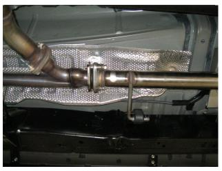
**Step 3.** You are now ready to install your new MAGNAFLOW system. Attach the the Inlet Pipe Assembly to the OEM Y-Pipe outlet using the existing hardware. Engage the welded hanber to the OEM rubber insulator. Leave all clamps and hardware loose for final adjustment of the complete system.
