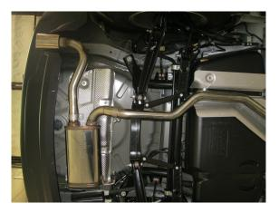
**Step 5.** Next use the supplied 2.25" clamps to attach the Muffler Assembly to the Mid Pipe and the Tail Pipe Assembly to the Muffler. Fit hangers into rubber insulators.
