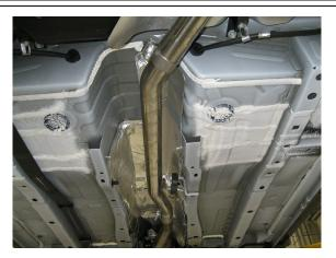
**Step 4.** Next use the supplied 2.25" clamp to attach the Mid-Pipe to the Inlet Pipe.
