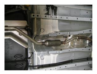
**Step 2.** Disengage hangers from rubber insulators and remove the OEM exhaust.
