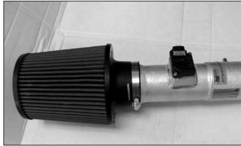
32. Install the K&N air filter to the intake tube, as shown.
