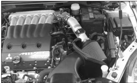
33. Install the Typhoon intake tube with the provided hardware, as shown. Adjust for best fit and clearance, then tighten all hardware, and hose clamps.
