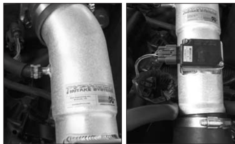
34. Reconnect the Crankcase vent hose and harness to the MAF sensor.
