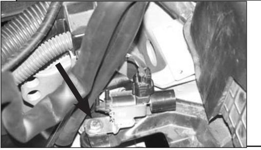
30. Reconnect the Vacuum Switching Valve Solenoid.
