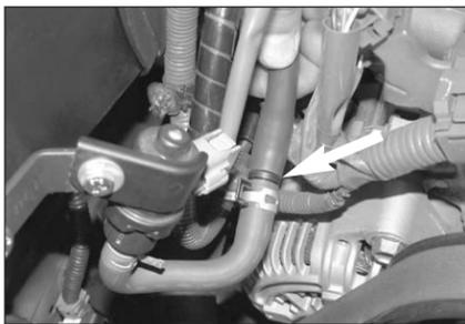
30. Connect the provided hose onto the evap solenoid as shown.
