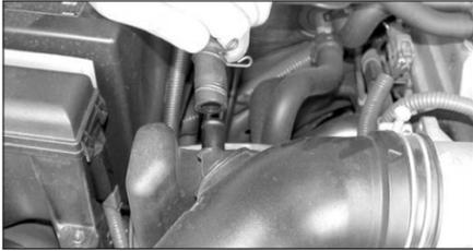
5. Remove the crank case vent from the intake tube as shown.
