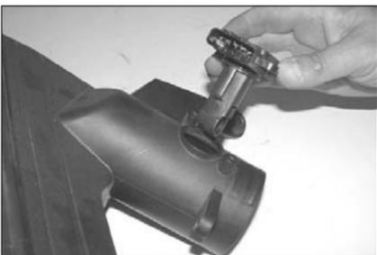
22. Remove the mass air from the factory air box as shown.
