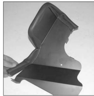
16. Install edge trim onto the heat shield as shown. Trim if needed.
