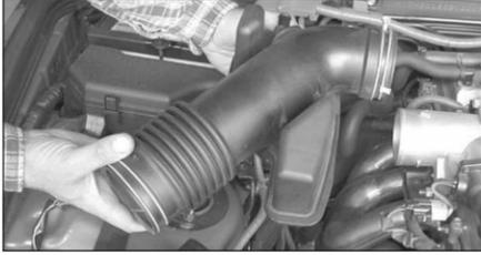
7. Remove the intake tube as shown.
