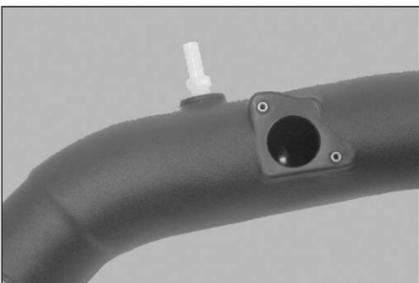
21. Install the vent fitting onto the new K&N intake tube as shown.
