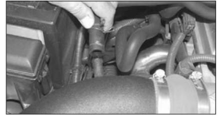
32. Reconnect the crank case vent as shown.
