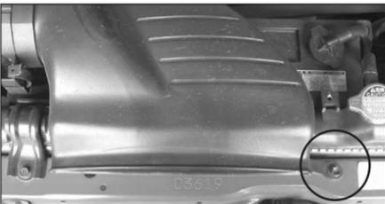
8. Loosen and remove the 10mm bolt that retains the fresh air intake to the vehicle then remove from the vehicle.
