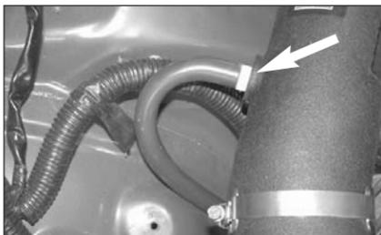
31. Connect the other end of the silicone hose onto the K&N intake tube as shown.
