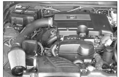
36. Re-install the engine cover with the factory hardware.
