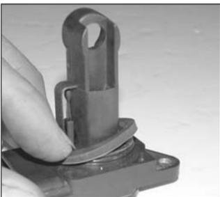
23. Install the provided gasket onto the mass air sensor with the sticky side towards the mass air.
