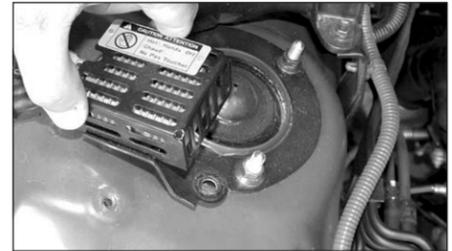
14. Loosen and remove the 12mm nut then lift and rotate relay box clockwise as shown.
