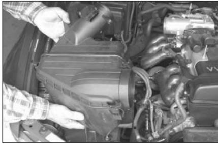
12. Remove the complete air box from vehicle.
