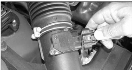
3. Disconnect the mass air electrical connection.
