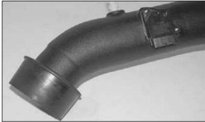
26. Install the filter adapter onto the K&N intake tube as shown.
