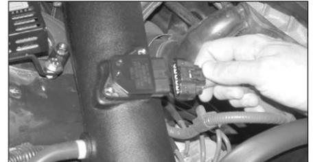
35. Reconnect the mass air electrical sensor as shown.
