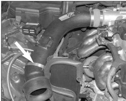
27. Install the K&N intake tube onto the throttle body and secure the tube to the saddle bracket with the provided hose clamp.
