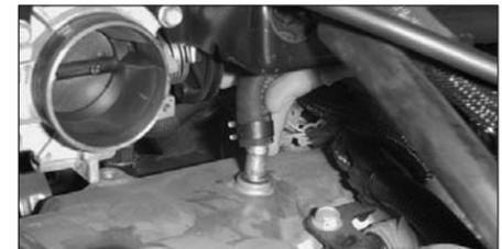
14. Detach the crankcase vent hose from the valve cover.
