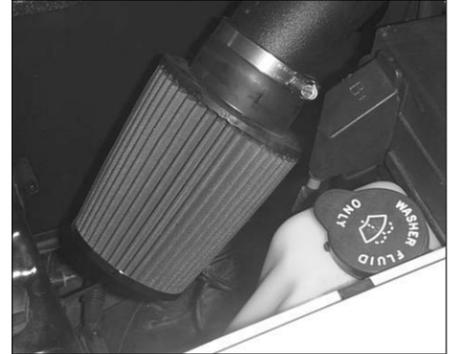
34. Install the filtercharger element and tighten hose clamp.
