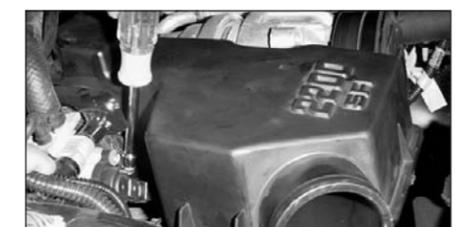
13. Loosen the hose clamp on the resonator at the throttle body.
