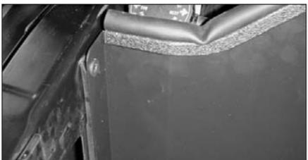
20. Secure the heat shield to the radiator core support using the clips removed in step 18.
