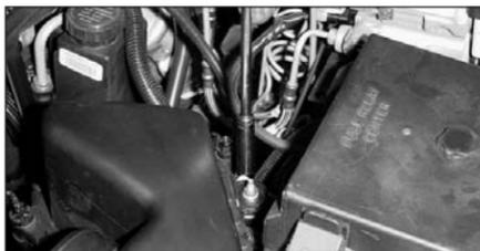
10. Loosen and remove the nut that retains the airbox to its mounting stud and remove airbox.
