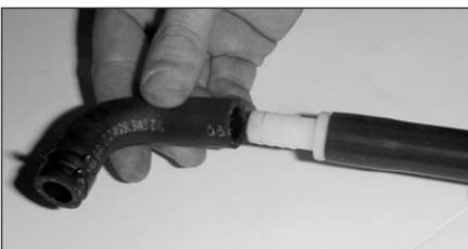
28. Connect the O.E. crankcase vent hose and vent hose provided using the hose mender.
