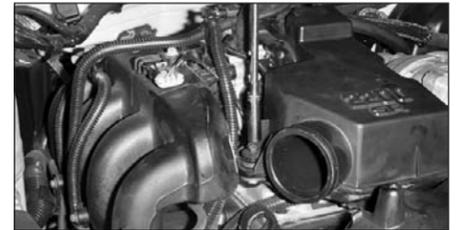
12. Loosen and remove the bolt that retains the resonator to its mounting bracket.
