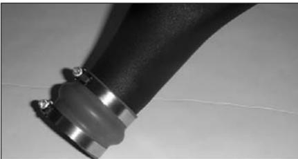
26. Attach the hump hose onto the K&N intake tube and tighten hose clamp.
