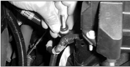
17. Install the 3/8"ID grommet onto the airbox mounting stud.
