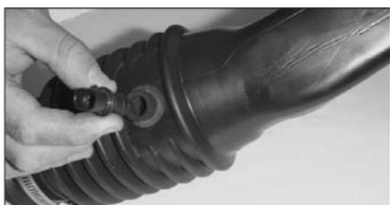
24. Remove the air temperature sensor from the stock intake hose.
