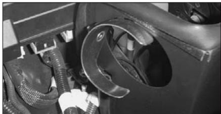
22. Install the saddle bracket assembly onto the airbox mounting stud and secure using the hardware provided.
