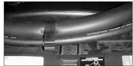
36. Secure the a/c lines to the radiator shroud with the retaining clip.
