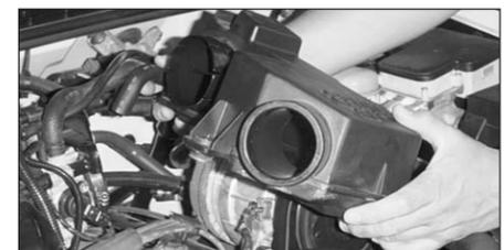
15. Detach the resonator from the throttle body and remove it.
