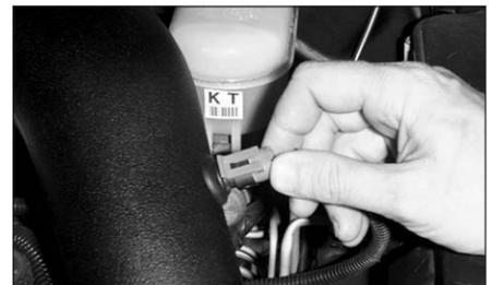
37. Reconnect the air temperature sensor electrical connection.
