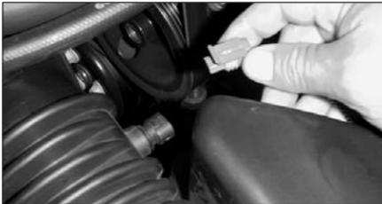
2. Disconnect the air temperature sensor electrical connection.
