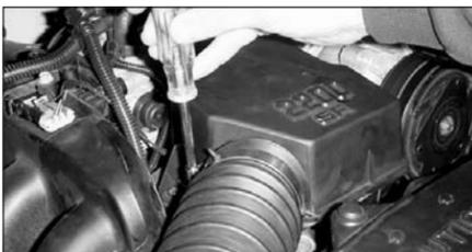
5. Loosen the hose clamp on the intake hose at the resonator.
