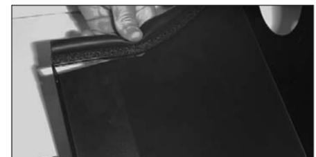
16. Install the trim seal onto the heat shield as shown.
