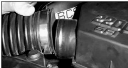
7. Detach the intake hose from the resonator.
