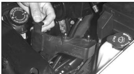
11. Press on the tab and lift and remove the airbox mounting bracket from the radiator core support.
