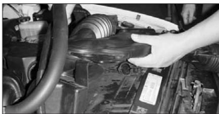
9. Remove the entire intake tube assembly.
