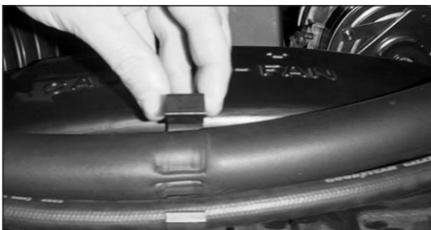
3. Detach the clip that retains the a/c lines to the radiator shroud.
