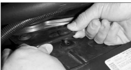
6. Pry up on the two push clips that retain the intake tube to the radiator shroud.
