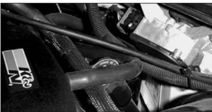
33. Attach the vent hose to the vent fitting on the intake tube.
