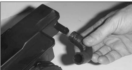
27. Detach the O.E. crankcase vent hose from the resonator.
