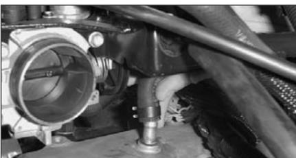
29. Attach the vent hose assembly to the vent fitting on the valve cover.
