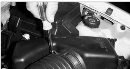
4. Loosen the hose clamp on the intake hose at the airbox.
