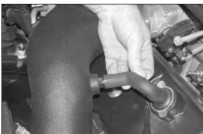
25. Install the crank case vent hose to the K&N intake tube.
