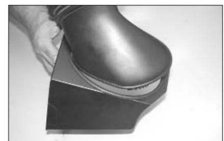
12. Snap the cold air duct removed in step 10 into the K&N heat shield as shown.
