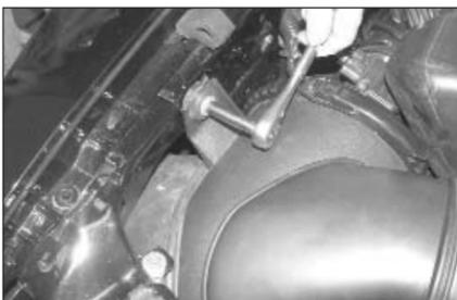
4. Loosen and remove the bolt that secures the air cleaner assembly to the inner fender.
