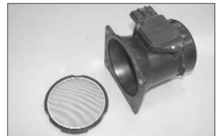
9a. Remove the diffuser screen from the mass air sensor.
