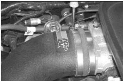
23. Secure the silicone hose to the throttle body using the hose clamp provided.
