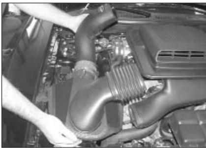
22. Install the K&N intake assembly, by sliding the bracket onto the protruding a/c line mounting stud as shown. Reconnect the fresh air duct to the hood scoop.
