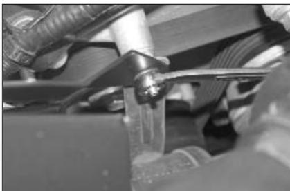
24. Secure the bracket to the a/c line mounting stud with the nut removed in step #20.
