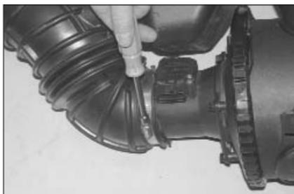
8. Loosen the hose clamp and detach the intake tube from the mass air sensor.
