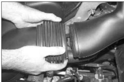
6. Separate the intake tube duct at fresh air intake inlet.
