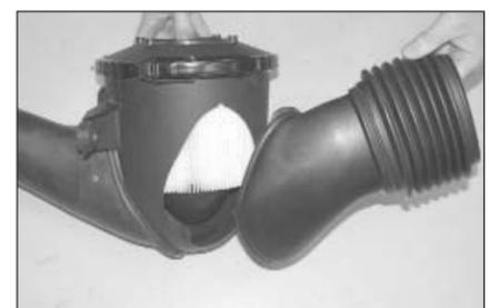
10. Separate the cold air duct from the airbox assembly.
