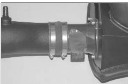
19. Attach the K&N intake tube to the mass air sensor using the hose clamp provided. **Note: Do not tighten completely at this time.**
