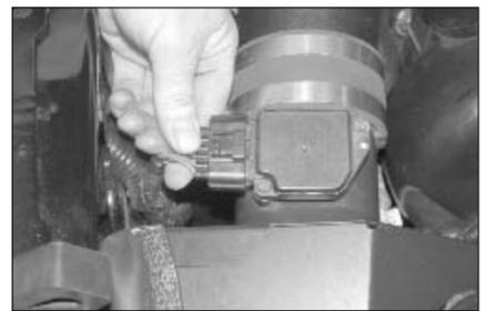
26. Reconnect the mass air sensor electrical connection.
