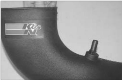
17. Install provided crank case vent fitting into K&N intake tube as shown.
