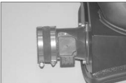
18. Attach silicone hose (08630) to the mass air sensor as shown.
