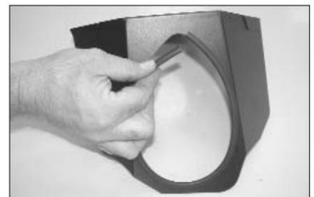
11. Install the 1/4 trim into the heat shield as shown.
