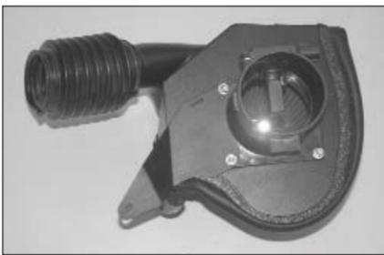
15. Attach the bracket to the mass air sensor as shown.
