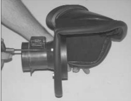
14. Assemble the mass air sensor, heat shield and adapter using the gaskets and hardware provided.
