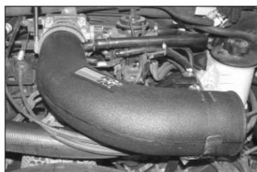
24. Install the K&N intake tube onto the throttle body, and tighten the hose clamp.
