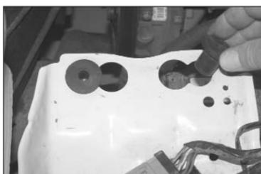
17. Install the two nut inserts onto the air box mounting tray as shown.
