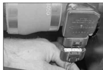
30. Reconnect the primary and secondary mass air electrical connections.
