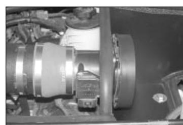
29. Attach the mass air assembly to the intake tube. Secure the mass air assembly and saddle bracket to the intake tube using the hose clamps provided.
