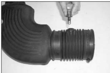
19. Remove the air temp. sensor from stock air intake tube as shown.
