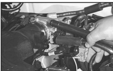
4b. On models with 5.4L, detach the idle air control and crankcase vent hose from the stock intake tube.
