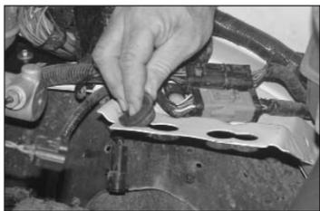
13. Remove the two air box mounting grommets from vehicle as shown.
