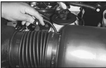
3. Disconnect the air temperature sensor electrical connection.
