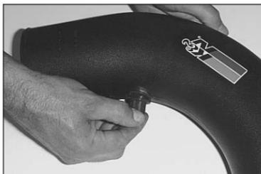
20. Using the grommet provided, install the air temperature sensor into the K&N intake tube.
