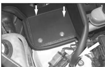
18. On vehicles with cruise control install heat shield as shown with the provided hardware.
