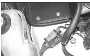
18a. On vehicles that did not come equipped with cruise control, install heat shield onto the vehicle, then secure with the provided hardware.
