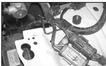
15a. On vehicles without cruise control, install the rubber mounted stud onto vehicle as shown.
