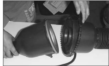
9. Open the air cleaner assembly and isolate the mass air sensor assembly.
