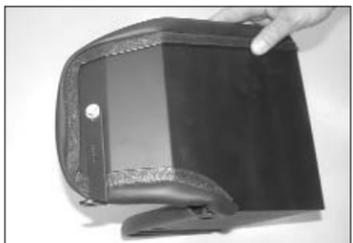
16. Install the provided "L" bracket (070952) onto heat shield as shown.
