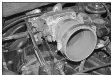
23. Using the hose clamp provided, attach the silicone hose (08724) to the throttle body.
