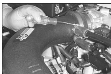
25. On models with 5.4L engines, install the idle air control and crankcase vent hose onto the appropriate fittings on the K&N intake tube, secure with the hose clamps provided.
