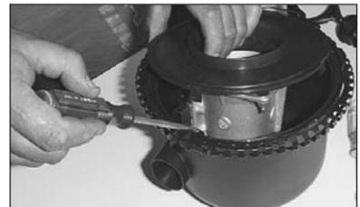
11. Using a flat blade screwdriver, push in and release the four clips that retain the mass air sensor retaining plate.
