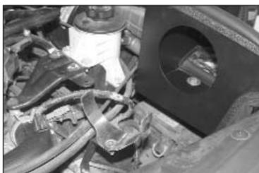
22. Install the saddle bracket assembly onto the protruding stud as shown, secure into place using the hardware provided.
