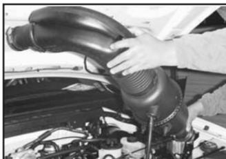
8. Remove the entire stock air intake assembly from the vehicle.
