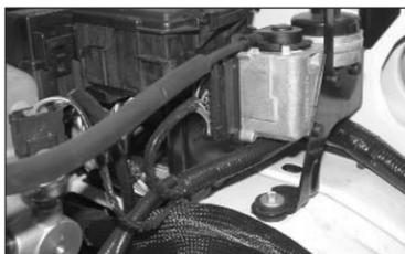
15. Remove the 6mm bolt that retains the cruise control onto vehicle.
