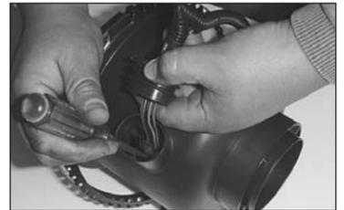
10. Slide the rubber grommet back and disconnect the primary mass air sensor electrical connection, using a flat blade screwdriver.
