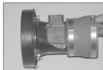
28. Install silicone hose (#08050) onto the mass air sensor with the provided hardware as shown.
