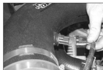
31. Reconnect the air temp. sensor electrical connection.
