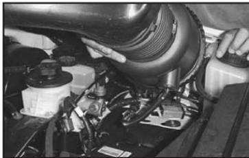
6. Detach the stock intake tube from the throttle body and lift up on the air cleaner assembly to release it from its retaining grommets.
