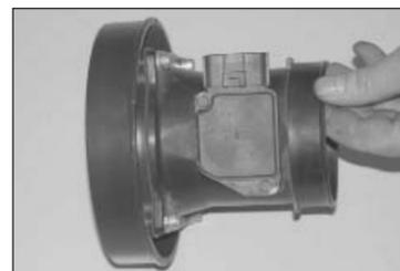
27. Attach the mass air adapter to the mass air sensor using the gasket and provided hardware.
