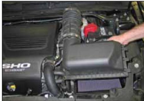
5. Remove the upper airbox/intake tube assembly from the vehicle.
