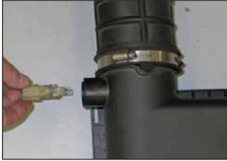
16. Release the locking tab on the inlet air temperature sensor and rotate counter clockwise to remove it from the factory airbox.
