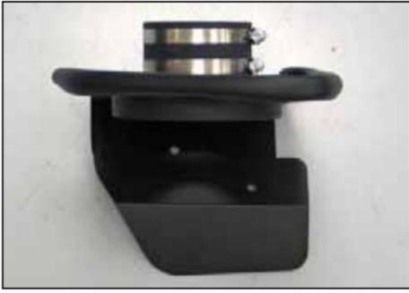
10. Install the provided silicone hose (08698) onto the filter adapter and secure with the provided hose clamp.
