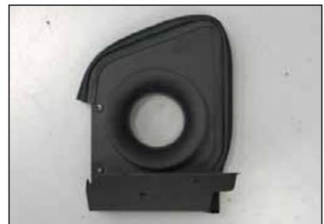
9. Install the filter adapter into the heat shield as shown and secure with the provided hardware.
