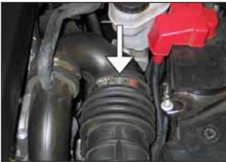
2. Loosen the hose clamp shown that secures the factory intake tube.
