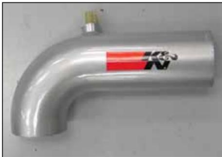
17. Install the inlet air temperature sensor into the K&N® intake tube and rotate it clockwise so it locks into position.
