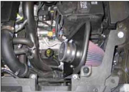
13. Install the heat shield/filter assembly into the vehicle so the mounting studs insert into the airbox mounting grommets.
