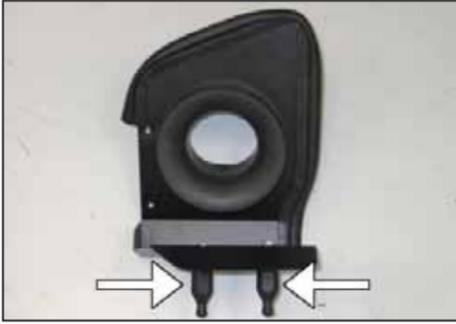
11. Install the two provided mounting studs onto the heat shield and secure with the provided hardware.
