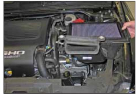
7. Lift up the airbox and remove it from the vehicle.
