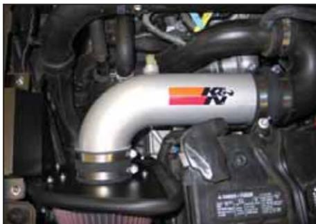
18. Install the K&N® intake tube into the silicone hump hose and then into the filter adapter's silicone hose. Secure the intake tube with the provided hose clamps.
