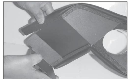
10. Install the edge seal to the heat shield as shown.
