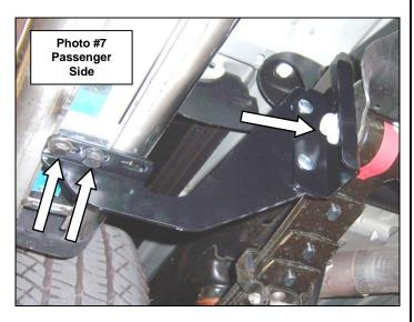
**Step-5** Re-align the side step with the vehicle and tighten all side bar, bracket and vehicle nuts and bolts. Repeat the installation steps to install the driver side brackets and side step. Remember to check and retighten all nuts and bolts periodically.
