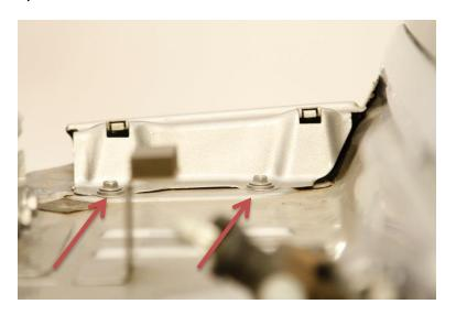
**4.** Bend the fender rounds back in order to gain access to the spot welds that hold the fender rounds to the fenders.
