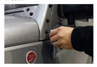
**2.** Remove the four button head torx bolts located in pairs on each side on the factory wiper motor cowl then remove the cowl center.
