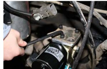
10. Once the mounting bolts have been tightened you can assemble the fuel line from the DDRP to the inlet of the factory fuel filter housing. Note: Early models will have the inlet/outlet ports on top of the filter housing (picture A), while later models will have the inlet port on the firewall side of the filter head (picture B).
