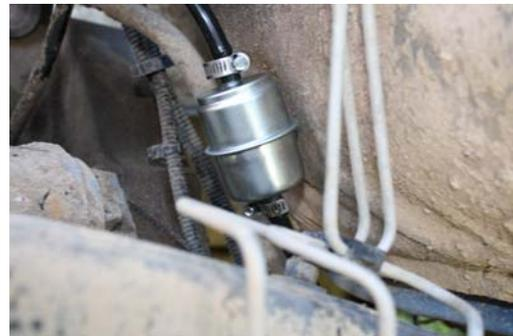
2. Remove the banjo bolt, located on the back side of the stock fuel pump. After removing the rear banjo bolt you must remove the fuel line retainer that attaches to the factory bracket. It is easier to remove the line on the back of the filter element before removing the final banjo bolt (this will save knuckles and o-rings).
