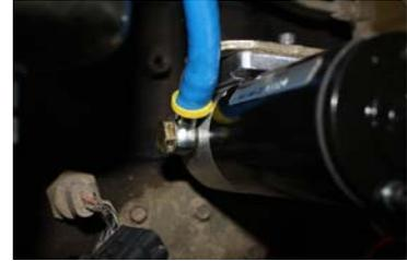
12. Measure and cut the opposite end of this fuel line to the inlet port of the factory fuel filter housing, top (early model) or top side (later model). Assemble into this port using the assembly instruction in the previous step.
