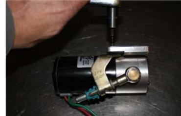
7. Using the 10 x 32 tapered flathead cap screw, locate the mounting hole of the support arm around this bolt while threading.
