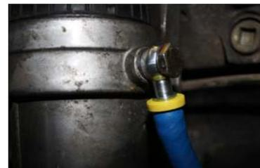
11. Spray WD-40 on the push lock portion of the banjo fitting and on the inside diameter of the fuel line before inserting the push lock into the fuel line. Assemble this banjo fitting to the outlet port of the DDRP using the banjo bolt and 2 washers.
