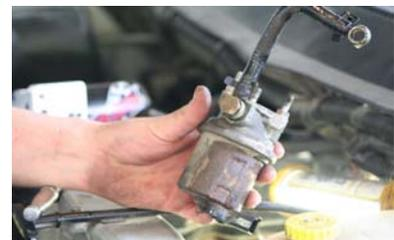
5. With the factory pump out of the truck you can remove the fuel line with the 17mm wrench.
