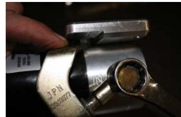
9. Now slide the DDRP into the factory location. Once the DDRP is in position use the included mounting bolts to bolt it in place.
