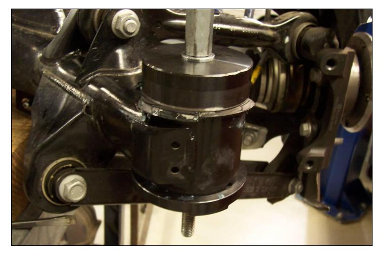
4. When you have all four of the new subframe mounts installed you can reinstall the subframe Assy in reverse order of removal.
